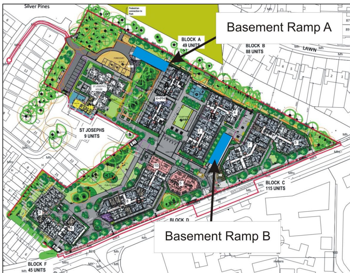
Figure 4.1 Proposed Vehicular Access Strategy - Dual Access from both Brewery Road and Leopardstown Road with double ramp to basement car park (Source: O'Mahony Pike Architects)
